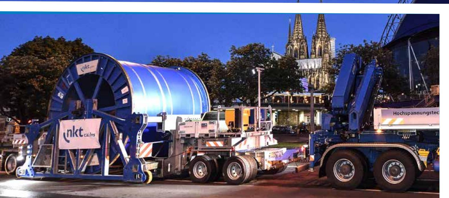
400kV ground cable on a 25 tonne drum being transported through Cologne, Germany. The cable made up part of the connection between a new gas and steam power plant and the German grid over a distance of 9 km - at present the longest 400kV ground cable connection in Germany
