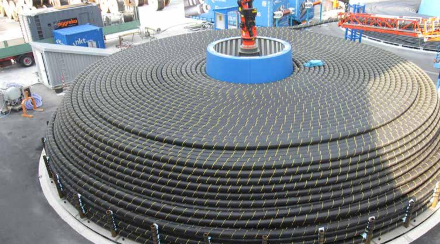
NKT Cables turntable with AC high-voltage offshore cables
